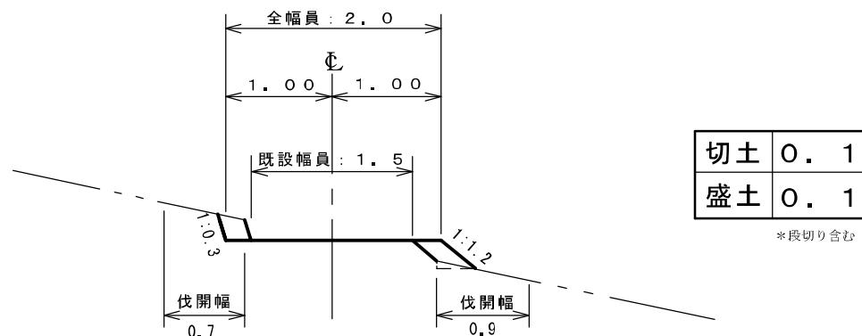
地山傾斜 = 30° ( $25^\circ \sim 35^\circ$ )
